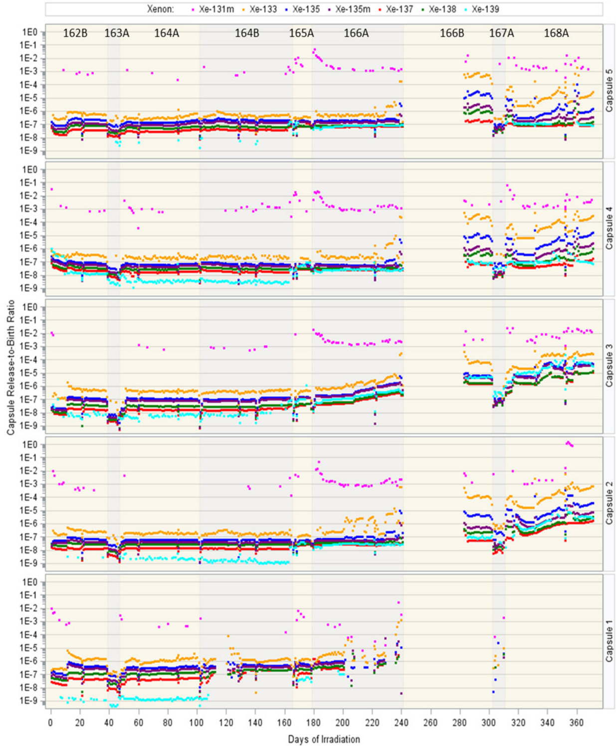
Figure 8. Measured R/B in AGR-5/6/7 capsules for xenon isotopes.
