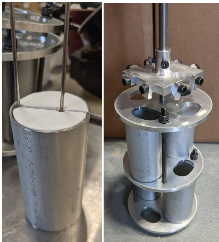
Figure 6. Photographs of a capsules and the experiment assembly prior to NaCl- \text{UCl}_3 capsule loading.
