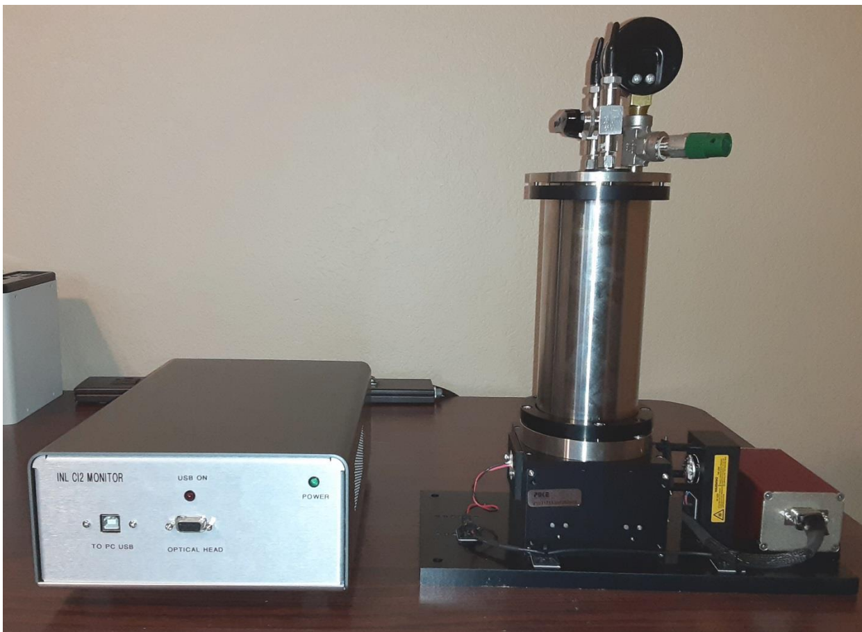
Figure 19: Custom Port City Instruments UV spectrometer for detection of \text{Cl}_2 gas at low concentrations.
