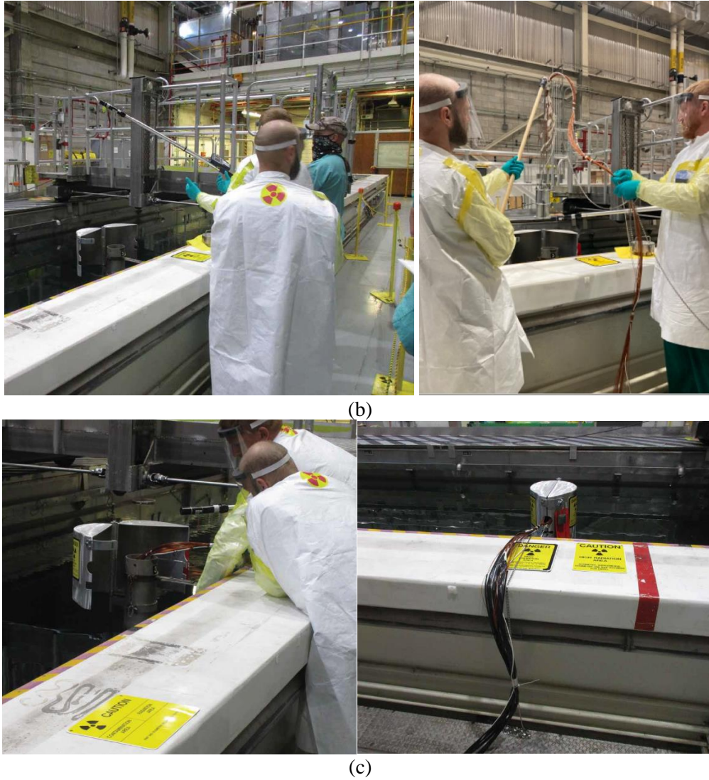
Figure 9. Photographs taken at ATR showing the process of inserting the salt capsules into the ATR gamma tube. (a) overall pictures showing the gamma tube and spent fuel pool with spent fuel assemblies at the bottom, (b) pictures showing engineers preparing the insertion of the salt capsules into the gamma tube, (c) pictures showing engineers inserting the salt capsules into gamma tube and gamma tube when the insertion of salt capsules is completed.
