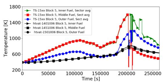
Measured (red, blue, green) and calculated (black) block temperatures from the nominal RELAP5-3D model
