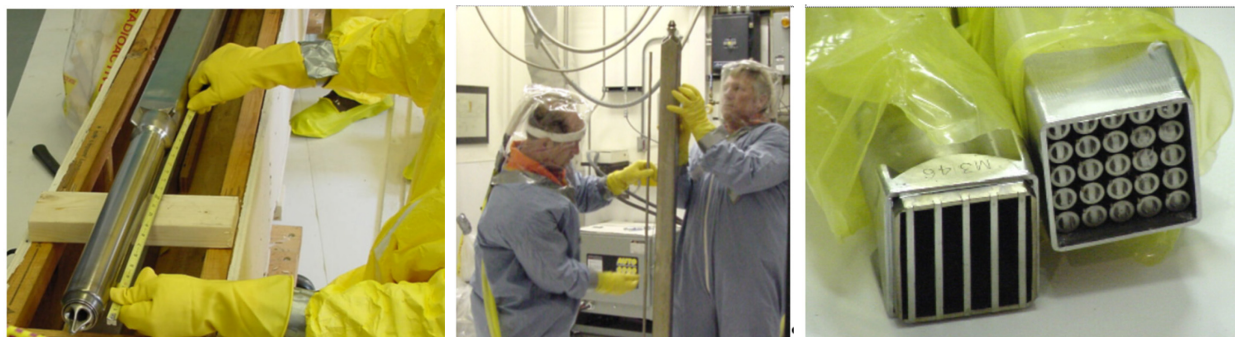
Figure 5. As received (left and center) and cut (right) unirradiated Fermi-1 radial blanket assembly, M346.
