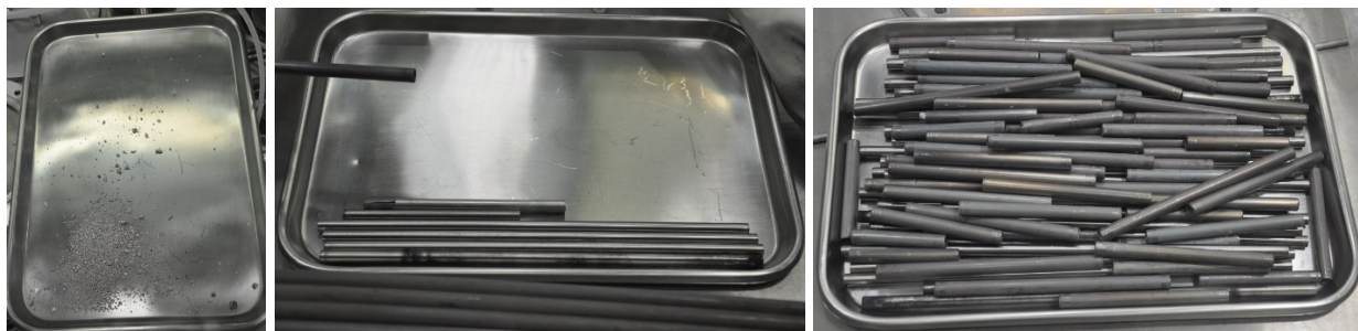
Figure 29. Steel tray used to collect loose sodium metal beads (left), the unloading of elements (center), and the sized cladding and separated slugs from five of the seven elements (left) in run 2.
