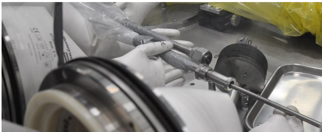
Figure 23. Loading of depleted uranium alloy slugs in LTC following MEDE run 1.
