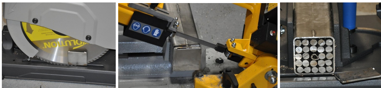
Figure 12. Cutting of mock Fermi-1 blanket assembly with chop (left) and band (center) saws, revealing cut end of assembly (right).
