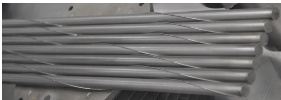
Figure 24. Fermi-1 radial blanket elements for MEDE run 2.
