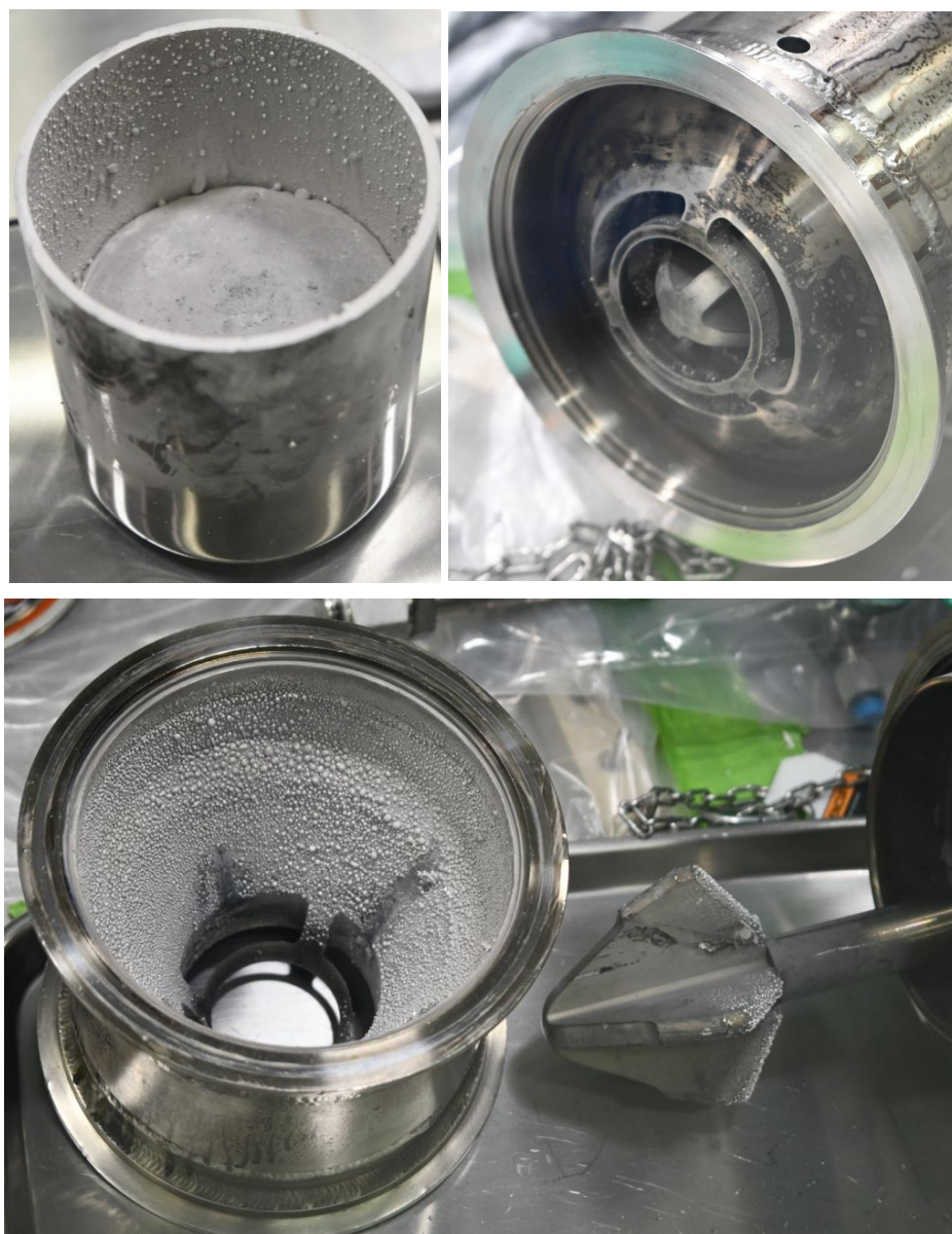
Figure 33. Post-run 3 crucible (upper left), underside of nickel funnel (upper right), top side of nickel funnel and push rod (bottom).
