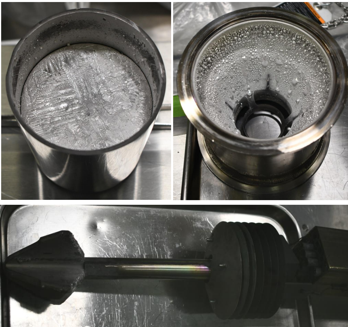
Figure 39. Post-run 4 crucible (upper left), top side of nickel funnel (upper right), and push rod (bottom).
