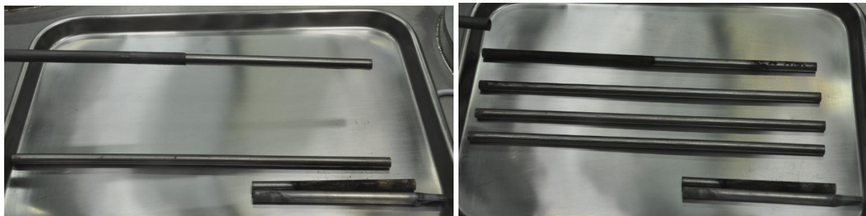
Figure 22. Post-run 1 depleted uranium slugs and cladding—during (left) and after (right) separation.
