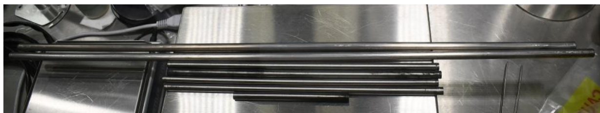
Figure 40. Removal of assembly from retort (left) and separated slugs from center element in the assembly following MEDE run 4.
