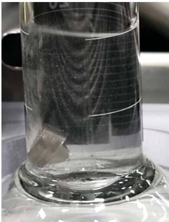
Figure 31. Bond sodium from the inner surface of a Fermi-1 radial element bottom end piece reacting in a graduated cylinder of ethyl alcohol.
