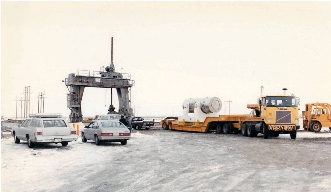
Figure 74. 125B cask on transport skid, loaded on trailer. (Courtesy NRC/INL tmi2kml)
