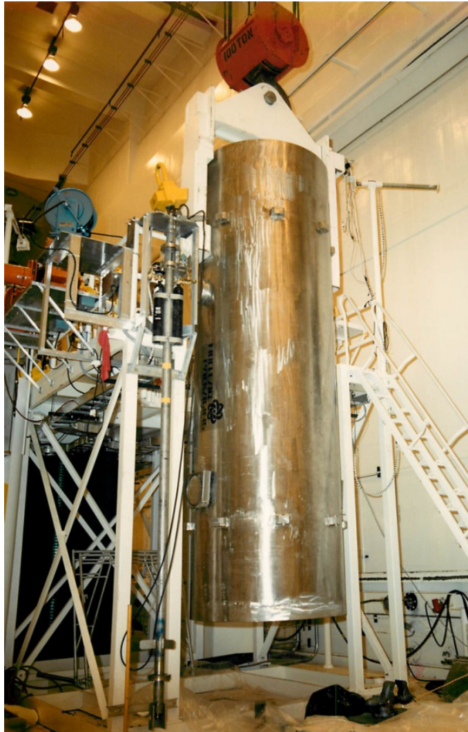
Figure 76. NuPac 125B cask on the work platform. (Courtesy NRC/INL tmi2kml)
