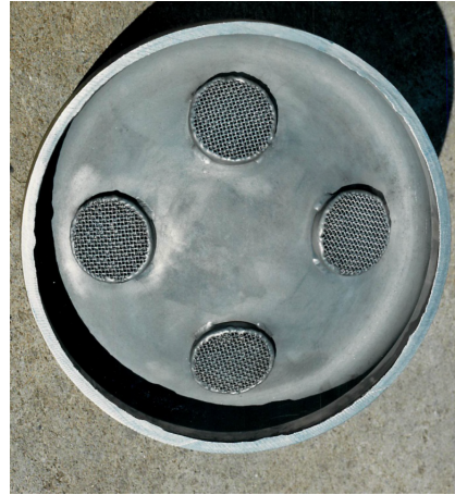
Figure 61. Cross-section view of fuel debris canister and lower head with catalyst bed. (Courtesy of INL, 2012)
