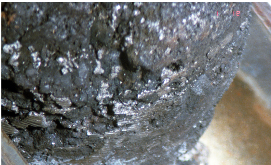
Figure 36 Core bore section consolidated melt material (Courtesy INL)
