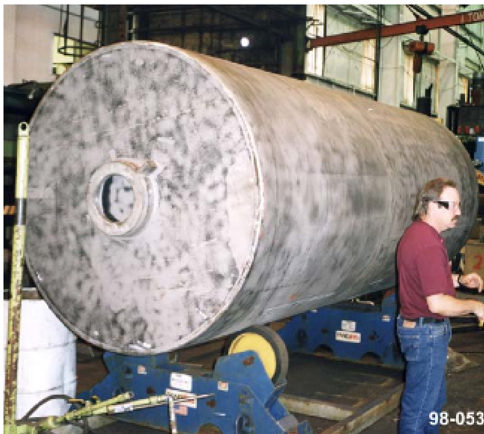
Figure 88. Photo of the DSC during fabrication. (Courtesy of INL)
