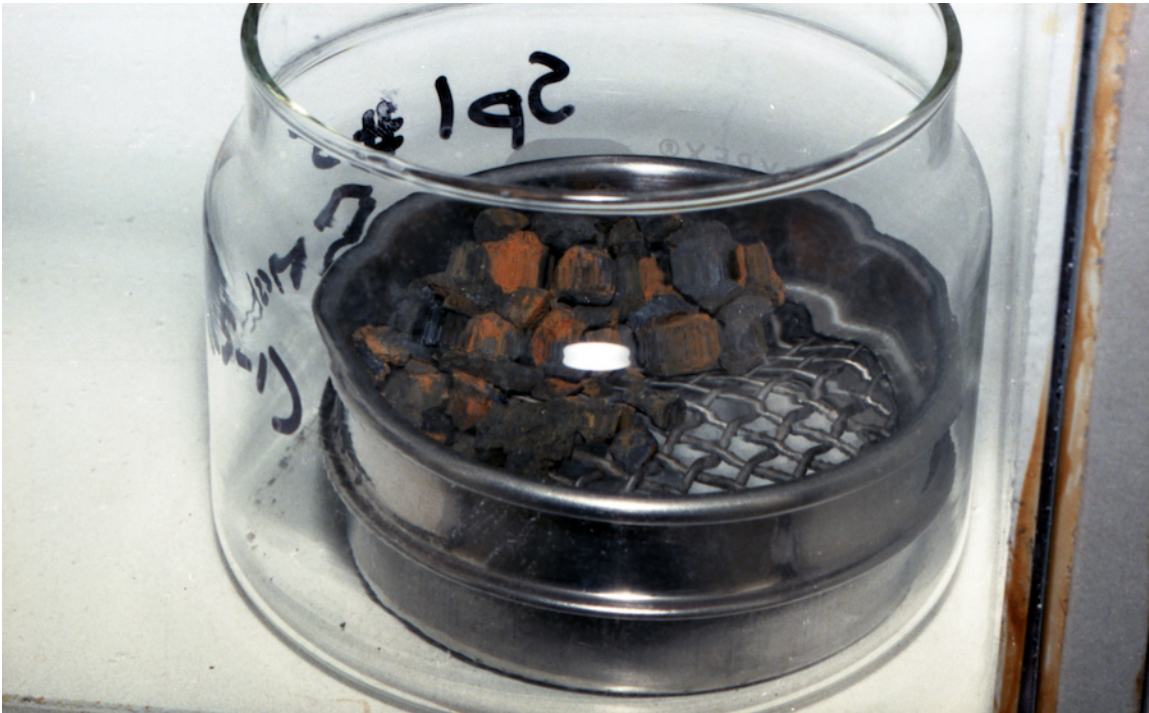
Figure 14. Loose material retained on sieve for size analysis. (Courtesy of INL, 1984)
