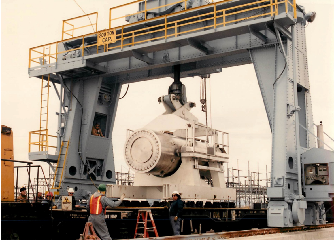
Figure 73. Gantry crane removing 125B Cask from rail car. (Courtesy NRC/INL tmi2kml)
