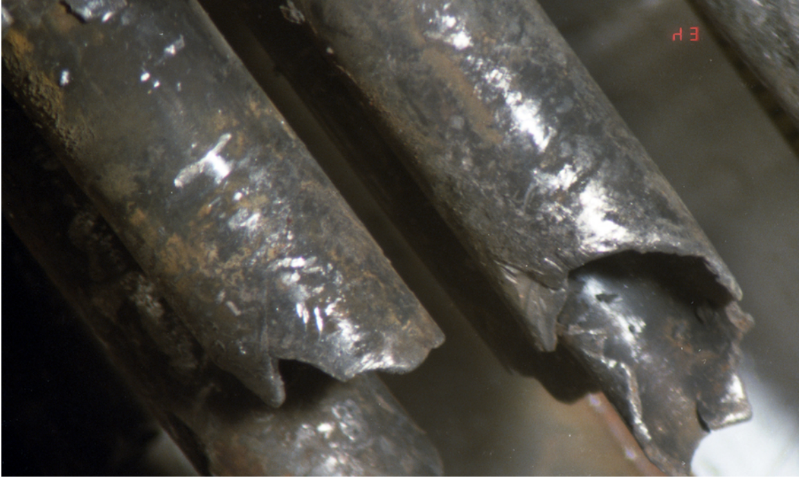
Figure 45 Rods Showing Discoloration and Melted Ends (Courtesy INL)
