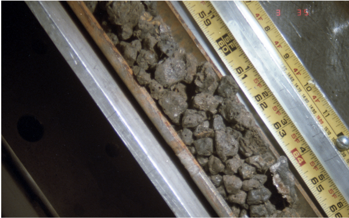
Figure 35 Core Bore Section with loose U-ZrOx gravel (Courtesy INL)
