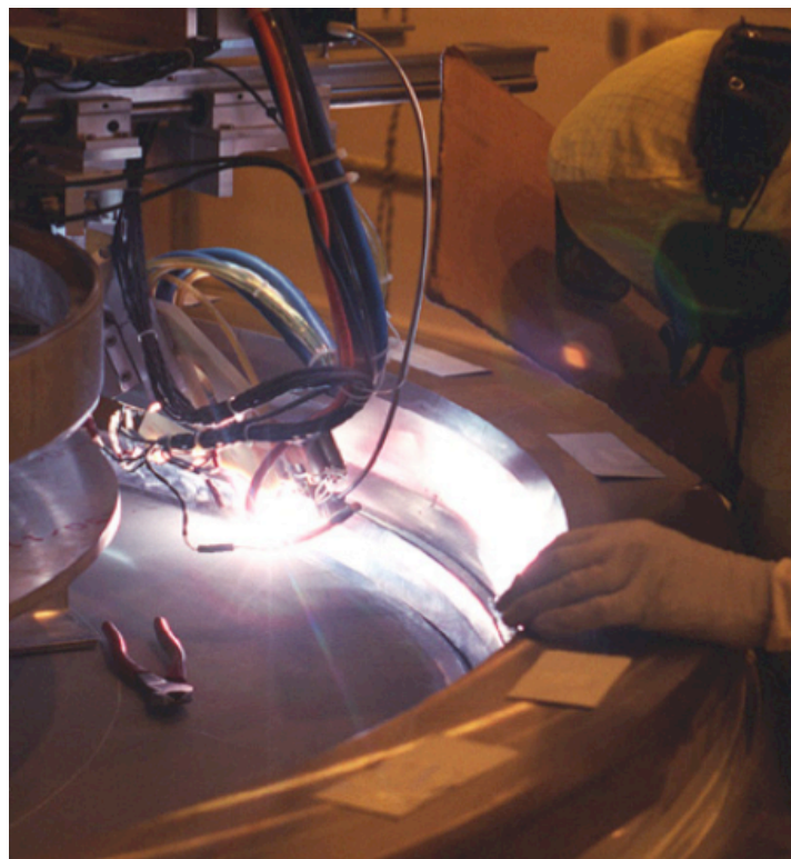
Figure 95. Welding of DSC lid. (Courtesy of INL)
