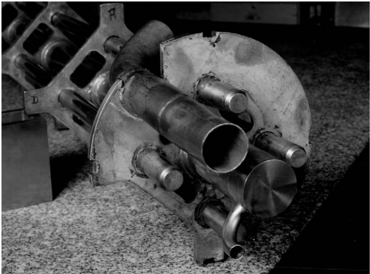
Figure 62. Internal structure of knockout canister. (Courtesy of INL, 2012)
