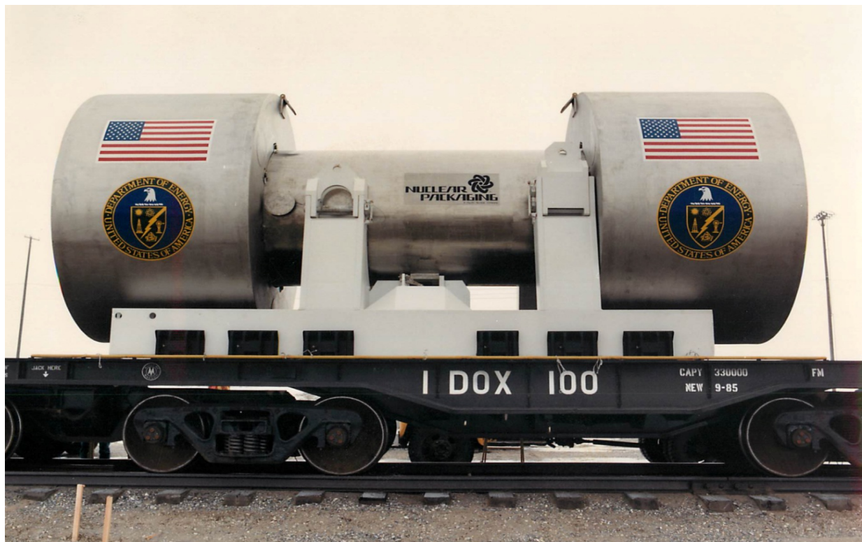
Figure 69. NuPac 125B cask on rail car. (Courtesy NRC/INL tmi2kml.inl.gov)
