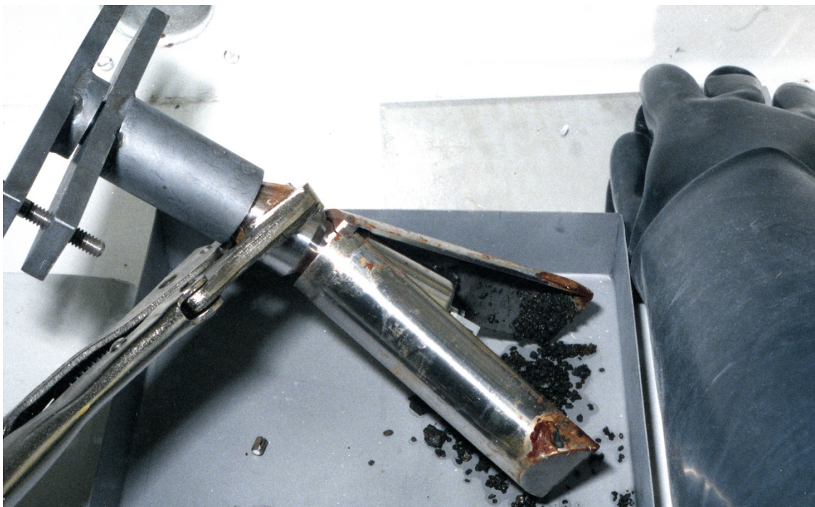
Figure 12. Clamshell Grab Sampler with Recovered Material. (Courtesy INL)
