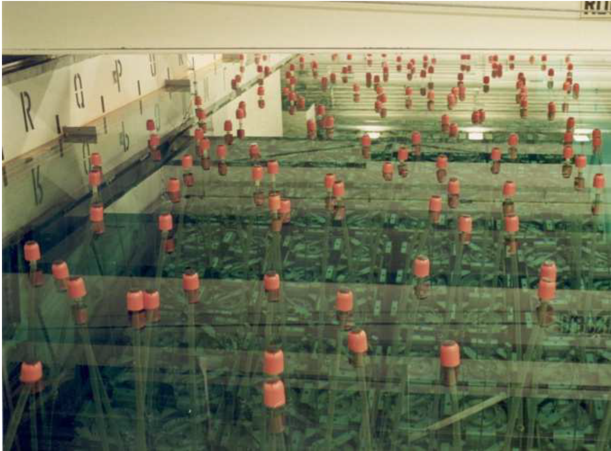
Figure 82. TAN-607 pool, showing six-pack racks and individual canister-vent ports (orange caps divert water back into pool). (Courtesy of NRC/INL tmi2kml)
