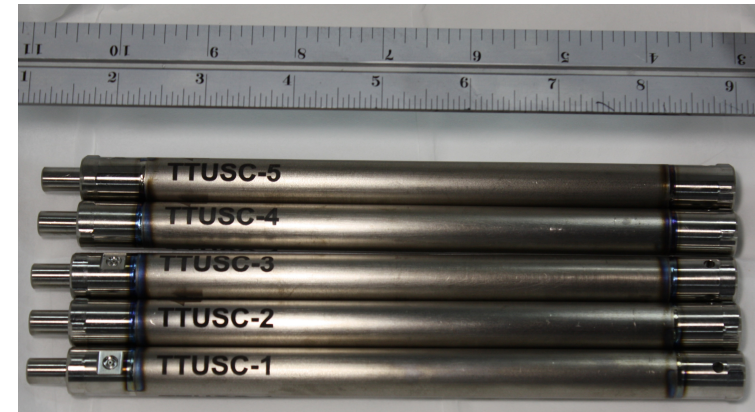
Figure 2. Capsules after final seal welding.
