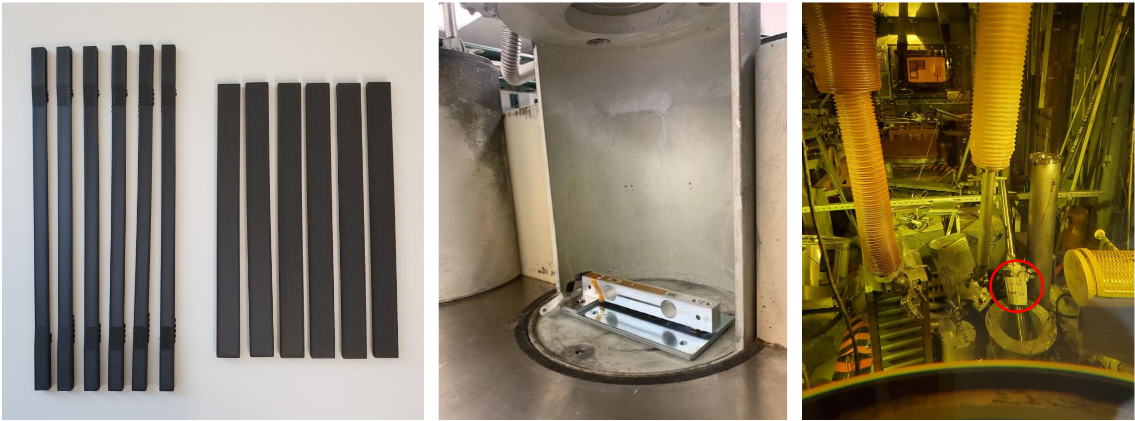
Figure 2: Left to right: CFR printed Tensile and Flexural samples, Cobalt 60 source irradiator, samples placed in the HFEF main cell (circled).
