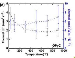
Thermal properties measurement of TRISO particle coatings from room temperature to 900 cusing laser-based thermoreflectance methods
