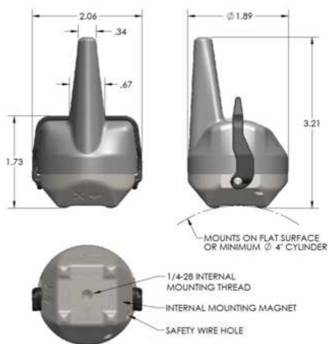
Figure 38. SD-VSN-3 sensor node dimensions.
