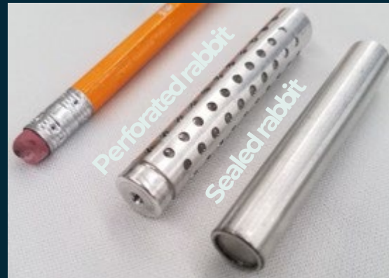
In-core liquid metal corrosion testing
