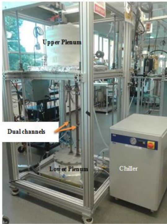
Figure 17. (a) Picture of P2PF preliminary design and (b) schematic diagram of P2PF preliminary design (all dimensions in inches). Adapted from [38].
