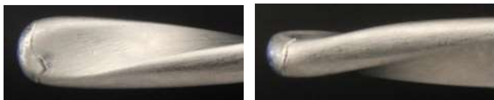
Fig. 7. Images of the detected non-compliance with the technical requirements of the nickel coating on the lateral surface of the fuel rods
