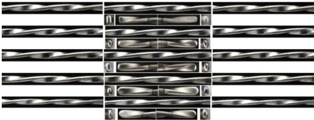
Fig. 5. Images of the appearance of the central sections and ends of fuel rods that complied with the requirements
