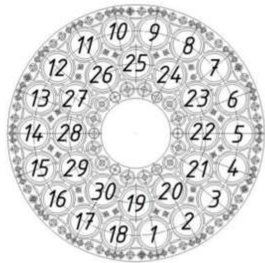
Fig. 2. Cartogram of the WCTC location in the IVG.1M reactor's core
