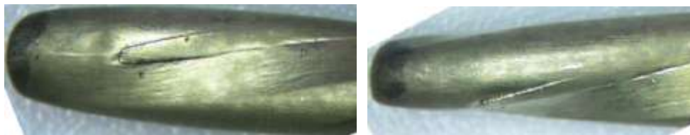
Fig 6. Images of the detected non-compliance with the technical requirements of the nickel coating on the lateral surface of the fuel elements
