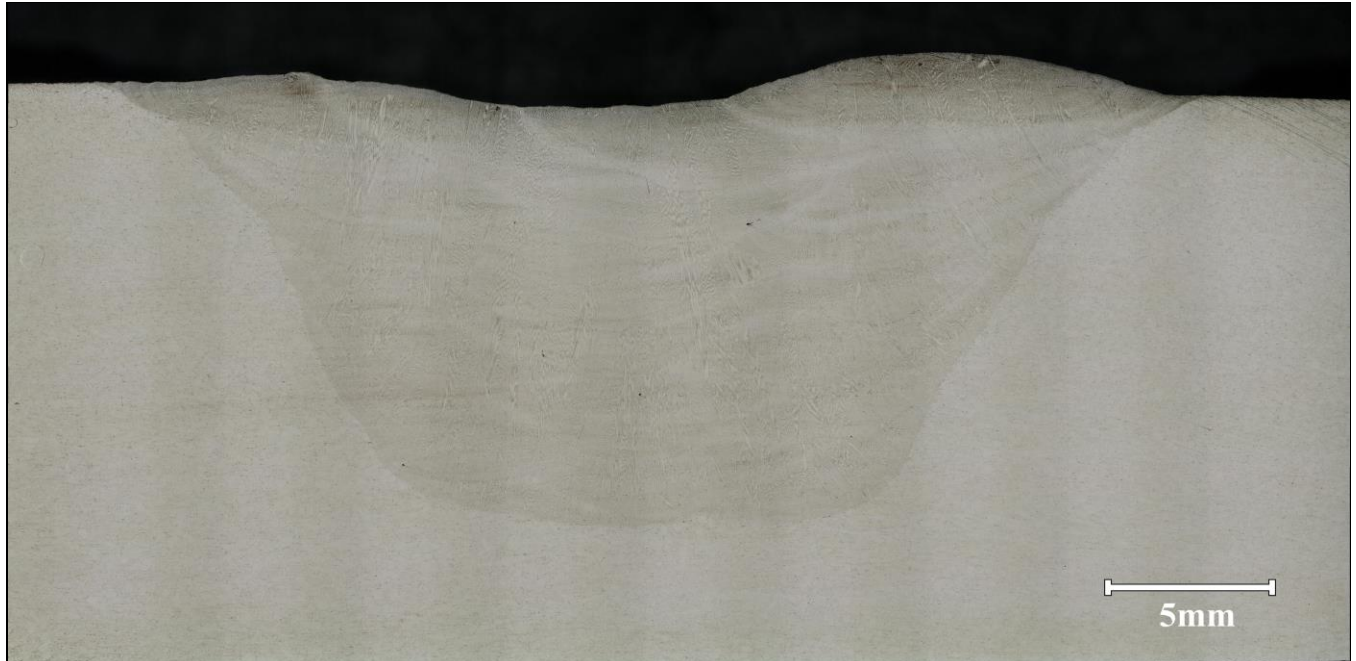
Fig. 7. First serial section of weld, Z11116, exhibiting a planar section without defects that would cause the weld to fail under the criteria of ASME Boiler and Pressure Vessel code, Section IX. (A few small pores are present but are not considered a failing defect according to the ASME code criteria.)
