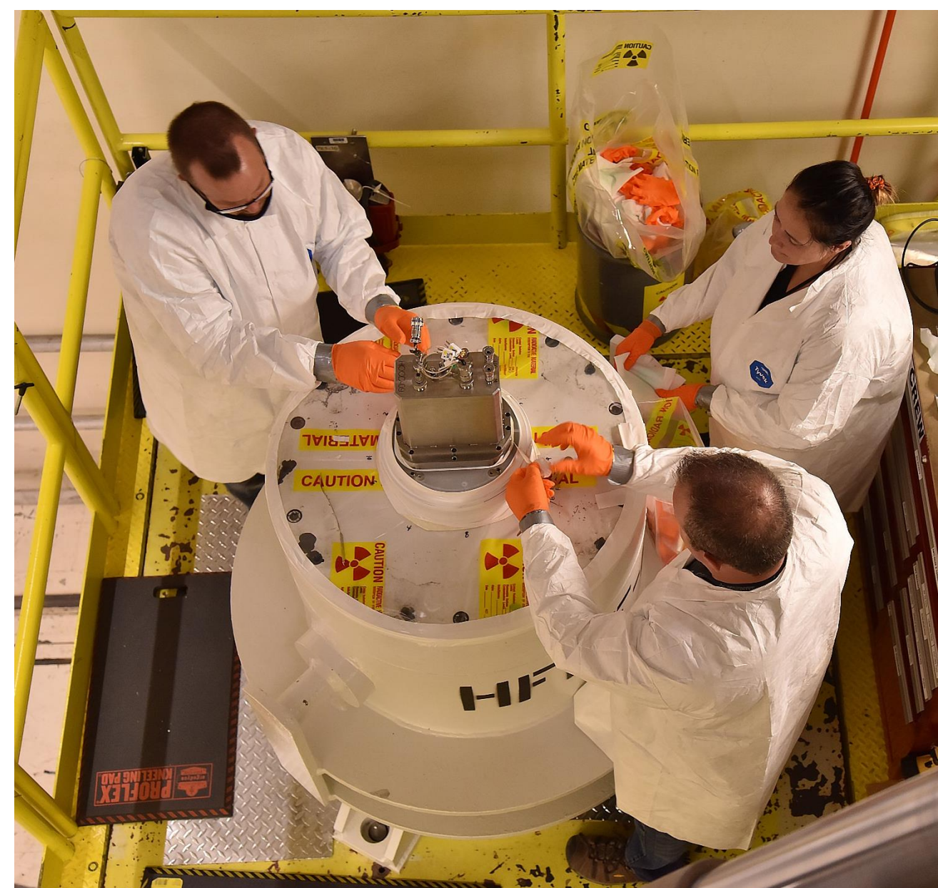
Final checkout in shielded cask, included instrumentation verification through hood and vehicle leak check
