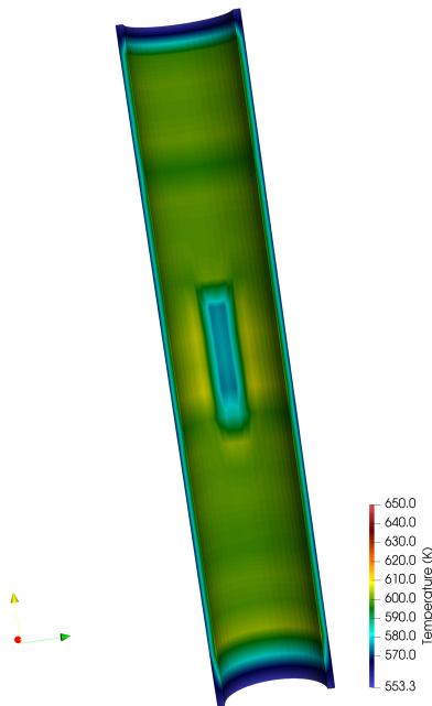
Figure 29: Temperature on cladding for a frictionless simulation.
