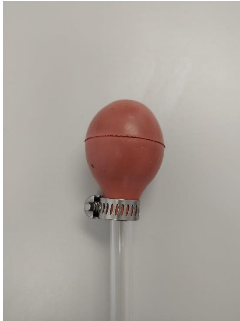
Figure 2. Rubber pipette bulb attached to quartz tube sampler.
