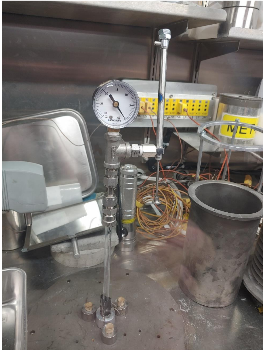
Figure 4. Filtered salt sampler with piston vacuum assembly in Molten Salt Furnace.
