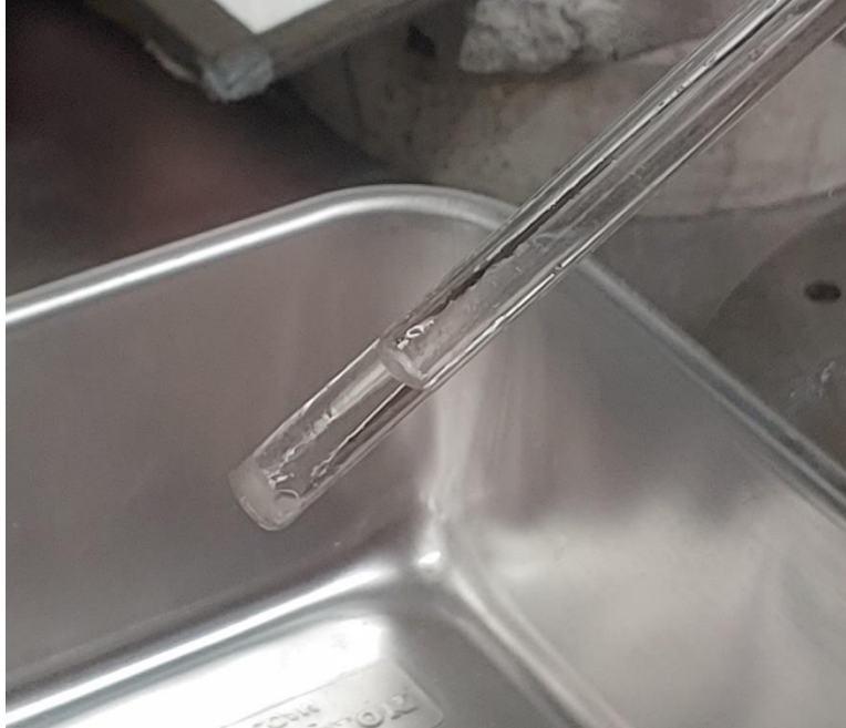
Figure 5. Molten salt sample taken with piston vacuum assembly.
