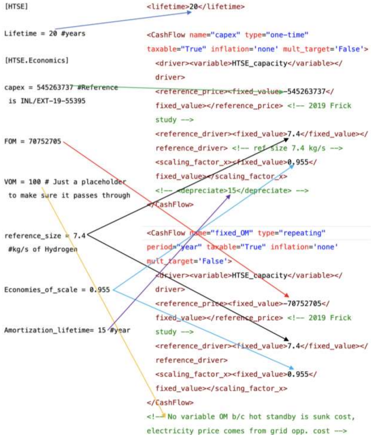
Figure 16. Manual information transfer between a HYBRID text file (left) and the HERON XML file (right).
