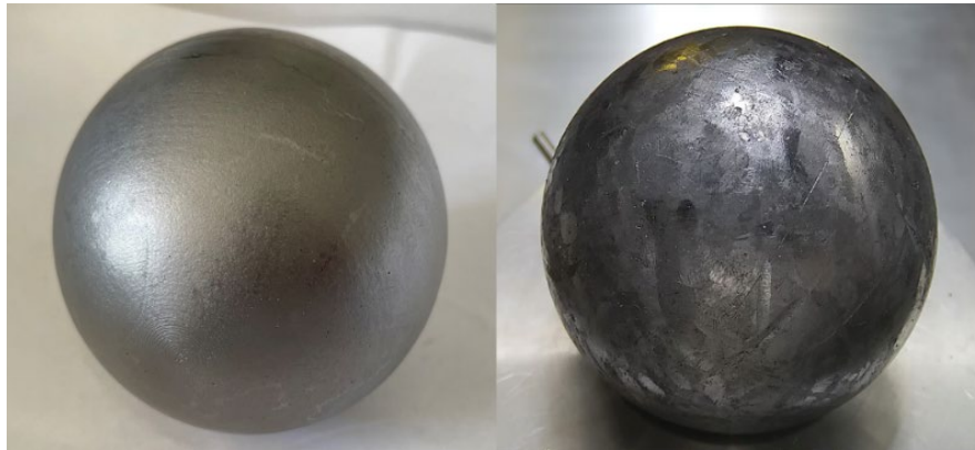
HTR fuels before (left) and after (right) irradiation
