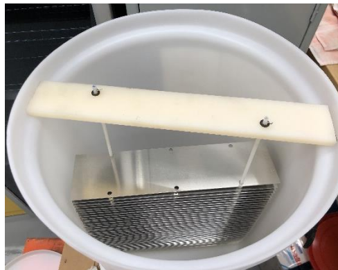
Figure 2. Plate corrosion assembly prior to immersion.
