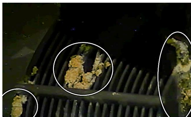
Figure 1. A closeup view of an INL ATR fuel element showing large, localized non-native corrosion plumes (highlighted by white rings) caused by a friction-type handling tool. Reproduced from reference 29.
