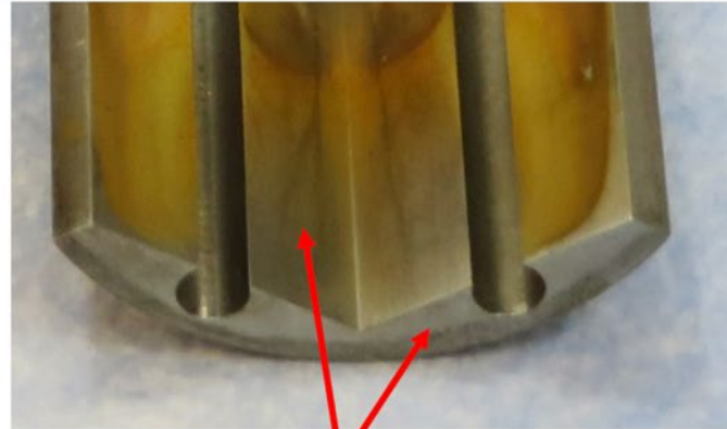
Yellow soot visible on inner wall of flask compared to silver/gray color of unexposed material
