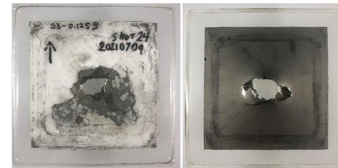
Fig. 2: Perforated bicomponent plate bonded with epoxy, front alumina ceramic (left) and rear Ti-6Al-4V plate (right).
