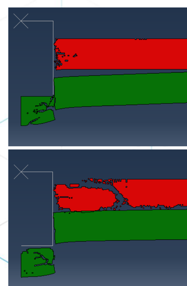
Fig. 3: Simulation of .50-cal FSP impacting alumina (red)/Ti-6Al-4V (green) plate using Abaqus/Explicit, stacked (top) and idealized bonding (bottom).
