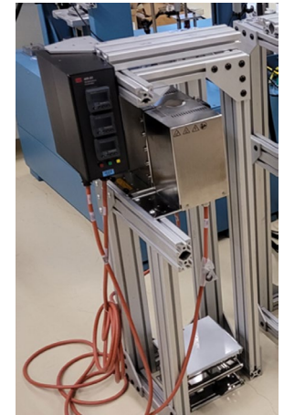
Fabricated in-cell creep frame.
