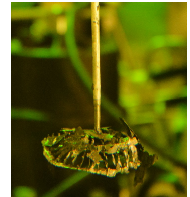
Robust iridium anode (A) and degraded platinum anode (B)
