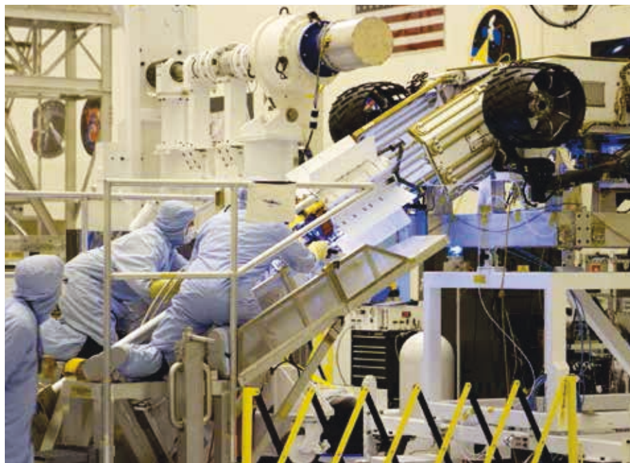
MMRTG being integrated to the Curiosity rover for testing in the Payload Hazardous Servicing Facility at KSC. (Photo: NASA)
