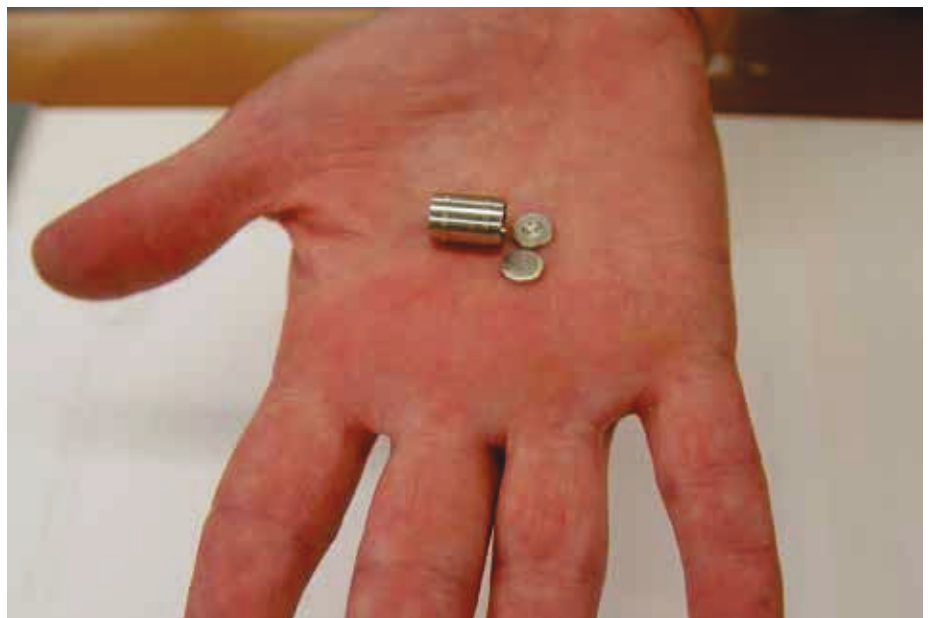
Lightweight RHU components. (Photo: ORNL)
