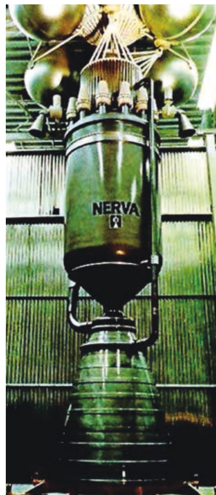
NERVA engine mockup. The spheres at the top contained hydrogen which, after passing through the reactor (center), was discharged out the nozzle (bottom of picture). (Photo: LANL Flickr)
