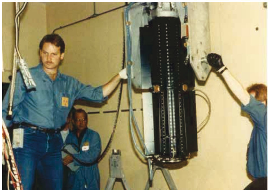
Mound technicians moving a GPHS-RTG in the vibration test cell using a crane on wheels. (Photo: Mound Museum Association)
