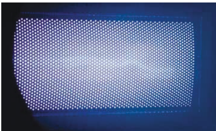
HiPEP thruster beam extraction test. (Photo: NASA GRC)
