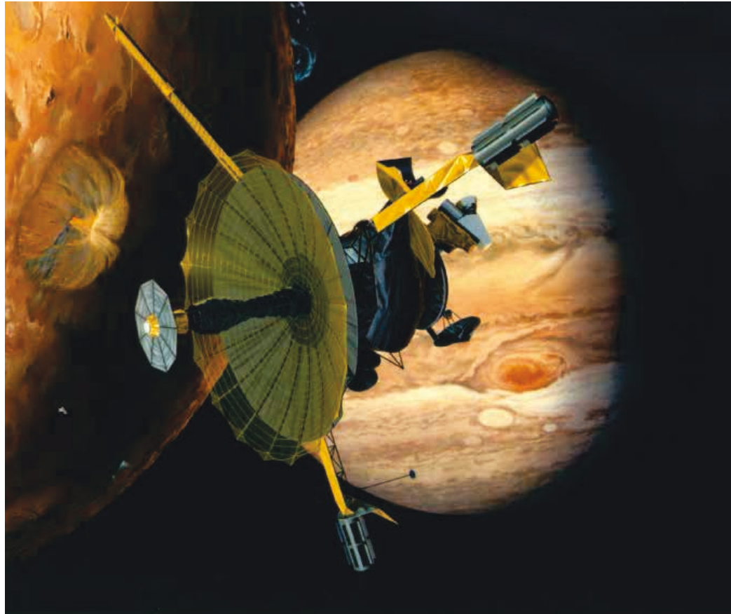
Artist's conception of the Galileo spacecraft. The GPHS-RTGs are located at the end of the booms on the back of the craft. (Photo: NASA.gov)
