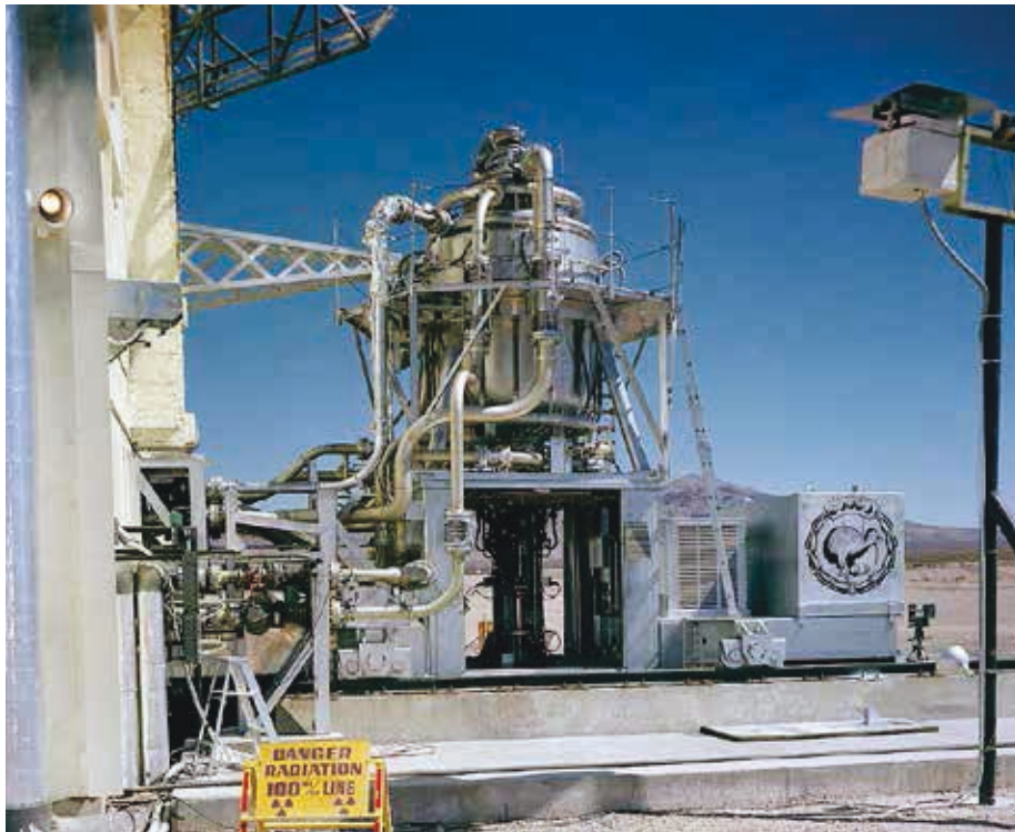
Kiwi-A reactor on a transfer cart. Note the Kiwi bird depicted on the side. (Photo: LANL Flickr)
