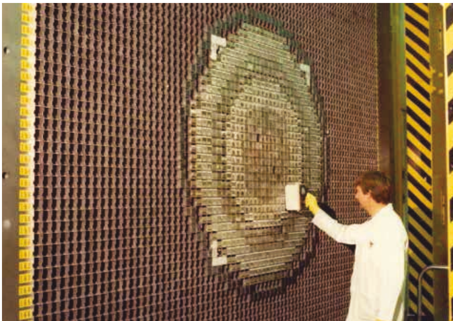
SP-100 core mockup in the ZPPR at ANL-W. (Photo: INL)
