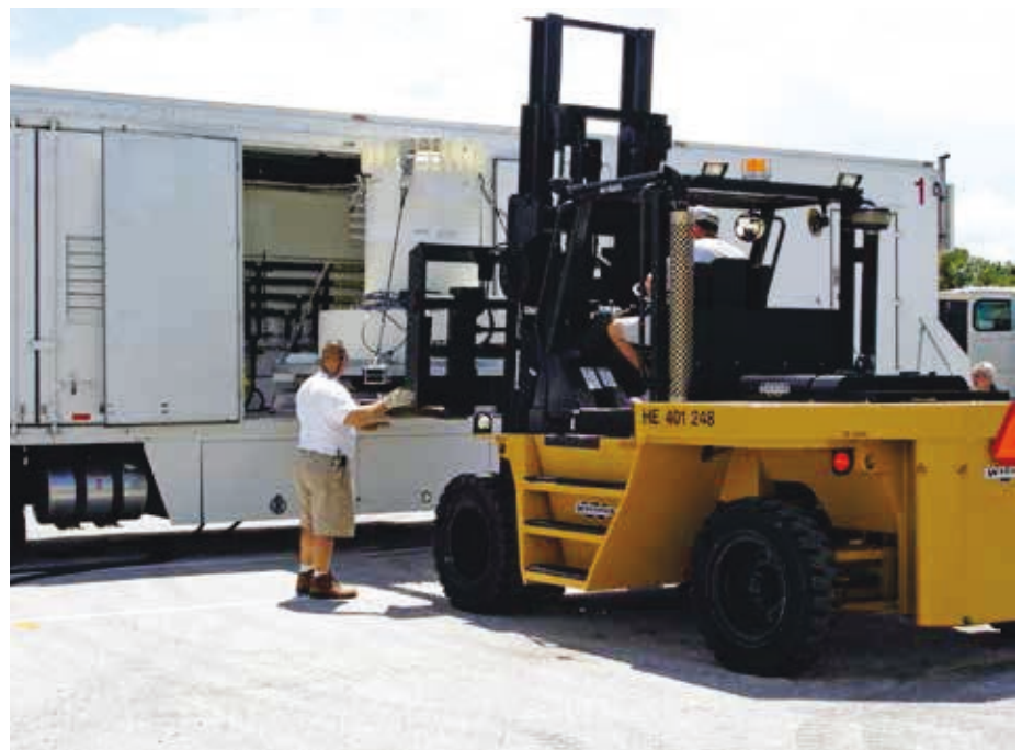
Operators remove an empty 9904 shipping package from an RTG transportation system trailer during training (circa 2005). The same system was used to move the Cassini GPHS RTGs from Mound Laboratory to KSC in 1997. (Photo: INL RPS Program)
