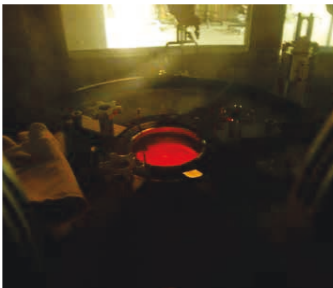
MMRTG assembly inside the SSPSF Inert Atmosphere Assembly Chamber. Clockwise beginning at top left. 1) Fueled GPHS modules being stacked. 2) The stack of eight GPHS modules ready for installation in the MMRTG housing. 3) The heated GPHS modules glow red inside the insulated MMRTG housing. 4) MMRTG assembly complete. (Photo: INL RPS Program)
