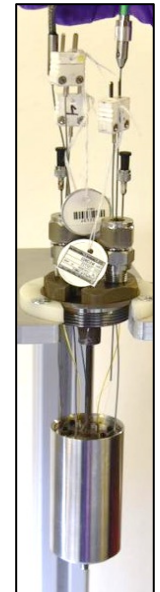
DRIFT-UO 2 capsule ready for insertion into a TREAT experiment vehicle
