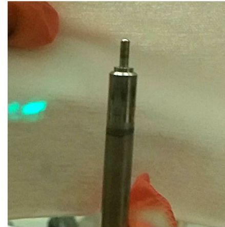
(a) Out of cell demonstration of endcap weld using REWS
