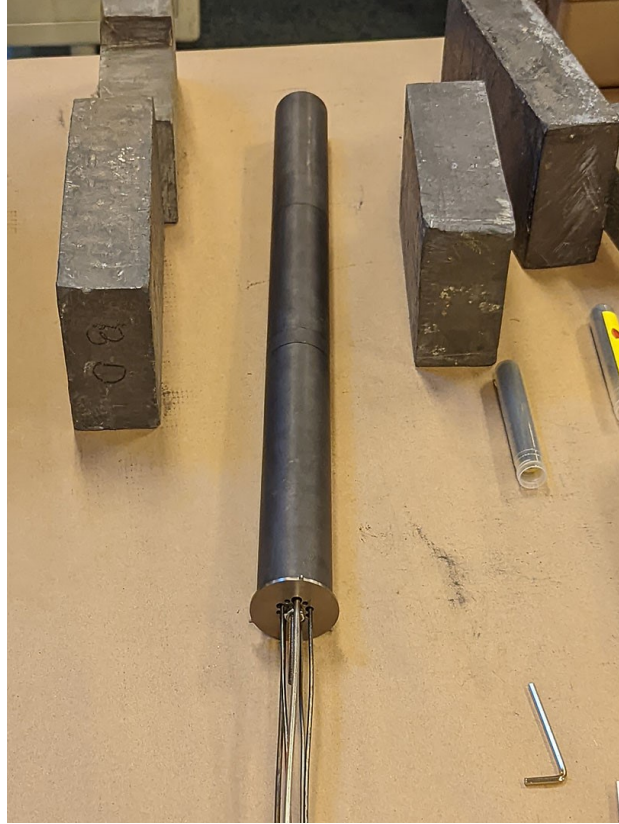
Figure 2. MITR capsule assembly with the tungsten alloy rod in the center position surrounded by sensors.
