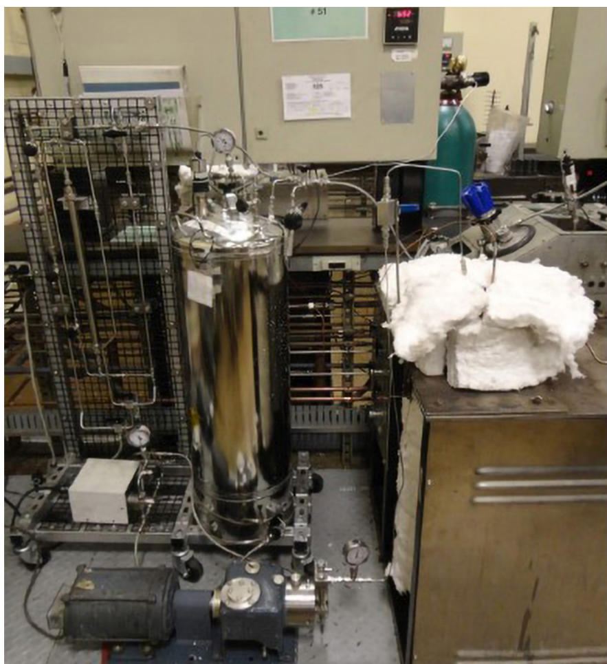
Figure 3. Test setup of 7.8 liter recirculating autoclave system at Westinghouse Churchill facility
