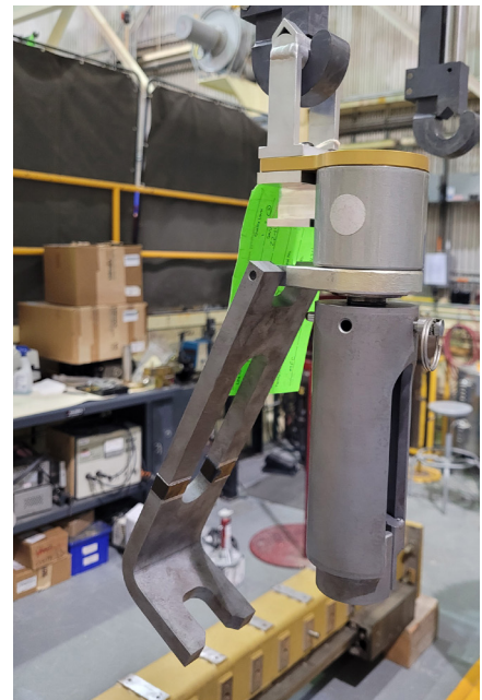
Figure 2. THOR capsule top cap torque multiplier used to seal the capsule at 120ft-lbf
