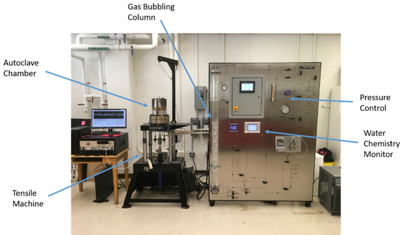
Figure 2. Autoclave setup for corrosion experiments at NCSU
