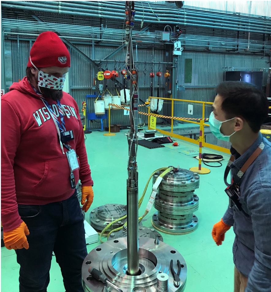
Figure 2. Final assembly of the THOR-C-2 capsule at the TREAT facility
