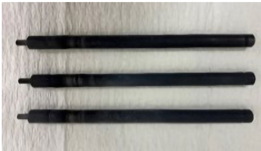
Figure 2. SiGA metal-bond rodlets with surrogate fuel molybdenum pellets delivered for ATR cycle
