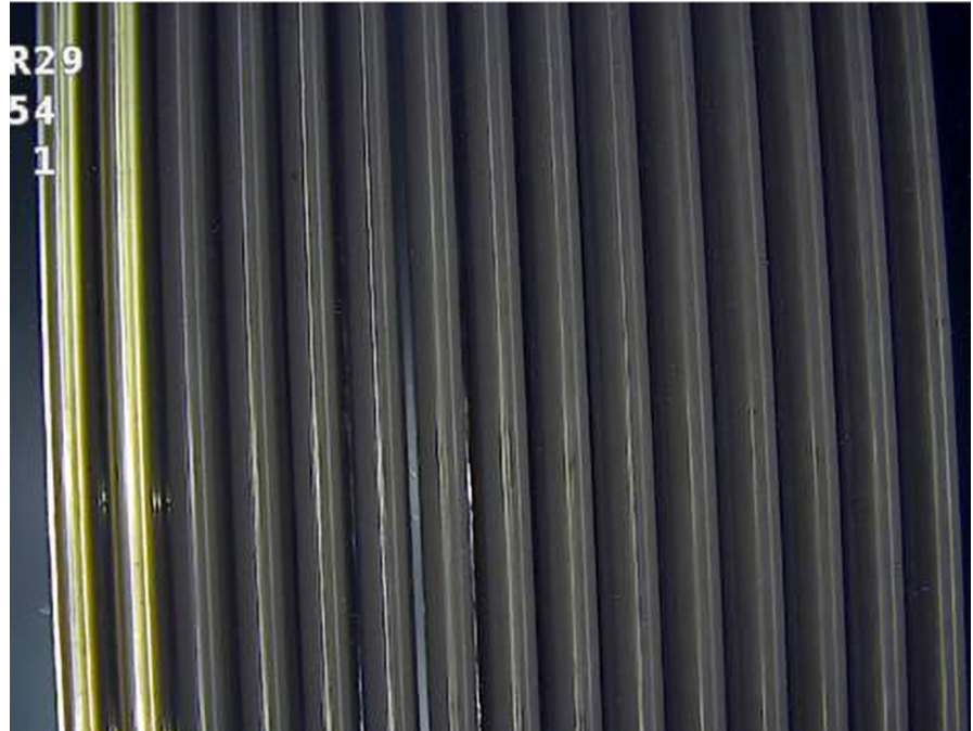
Figure 3. Cr-coated fuel rods after one cycle in ANO (two corner rods on left were coated with chromium)
