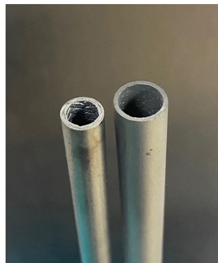
Figure 1. Comparison of smaller diameter and standard ATF diameter SiGA® cladding
