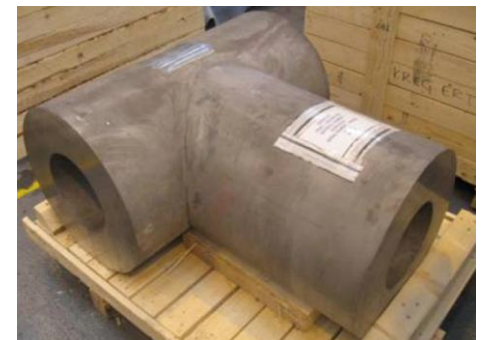
316L PM-HIP component for ASME Section III Code Case N-834
