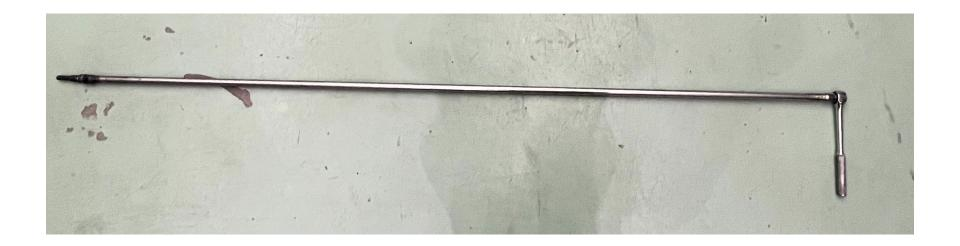
½ inch hex/allen socket welded to an 81 inch long reach tool and socket wrench
