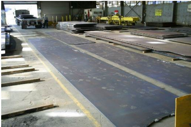
Photograph of first commercial heat A709 plates in as-rolled condition
