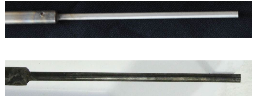
Ru anode before (top) and after (bottom) the electrolytic reduction of 200 g of uranium oxide.
