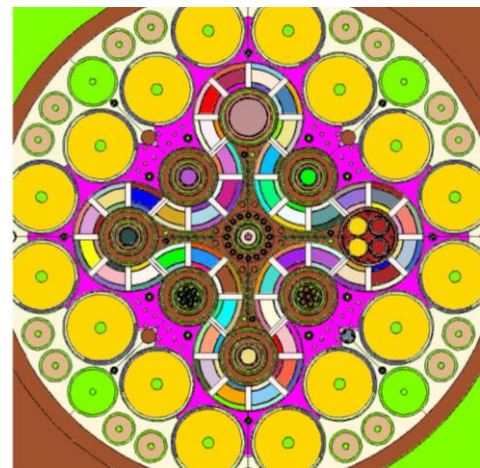
Fig. 2. MCNP cross section of the ATR.
