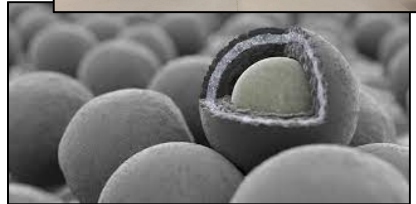
TRISO fuel particle showing protective layers of carbon and silicon carbide on a uranium oxycarbide fuel particle.
