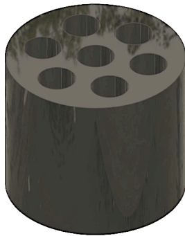
Fig. 3. Three-dimensional rendering of a single SIRIUS-3 fuel specimen
