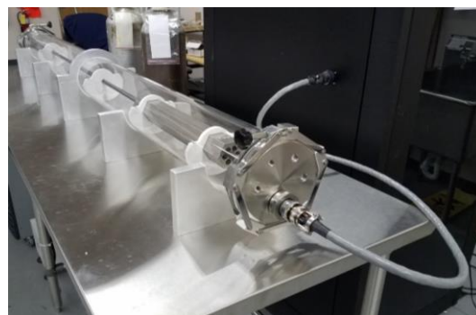
Fig. 3. Single heat-pipe experiment quartz tube with core block, end flange, and Macor ceramic supports.
