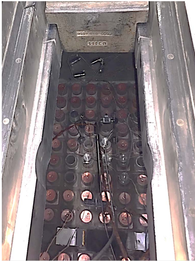
Figure 1. Testing of in-core sensors at TREAT. (Left) Top view of the TREAT core assembly, loaded with instruments and showing lead wiring. (Right) Example data results from instrumentation testing in TREAT. The top plot compares data collected from a Gd-SPND to the measured reactor power. The bottom plot shows the axial core temperature measurements taken by a distributed temperature optical fiber sensor.
