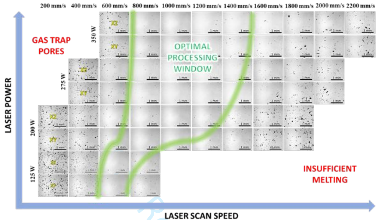
Figure 5: Optical micrographs of XZ and XY cross sections of IN718 samples produced with varying laser power and laser scan speed, while hatch spacing ( 120\ \mu\text{m} ), and slice thickness ( 30\ \mu\text{m} ) were kept constant.
