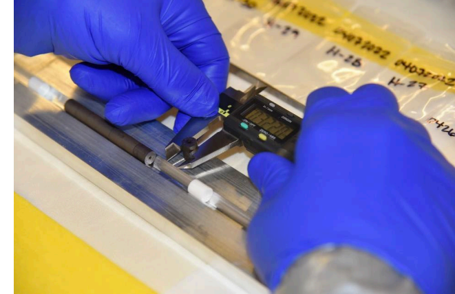
Rodlet internals and a fuel pellet dimension.
