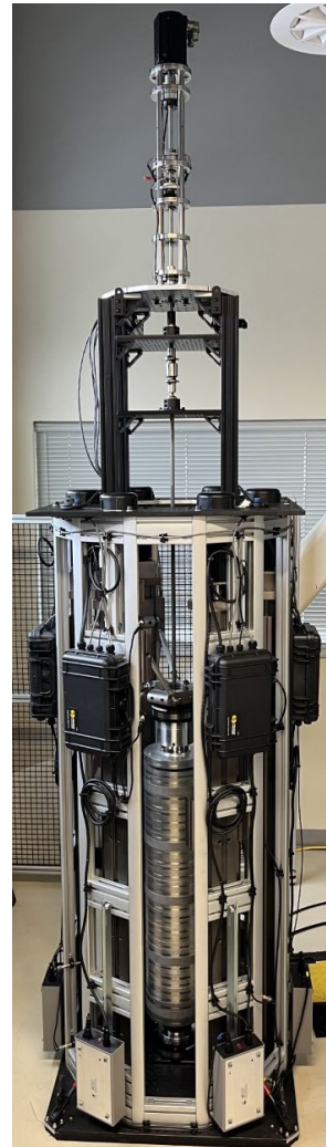
MARVEL Control Drum Prototype in ASI Double Delta Platform.
