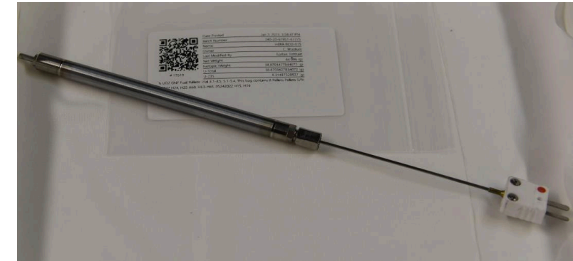
Completed rodlet assembly with cold spray Cr-coated zircaloy.
