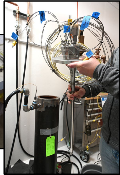
Installing the prototype irradiation vehicle in the out-of-pile test rig.
