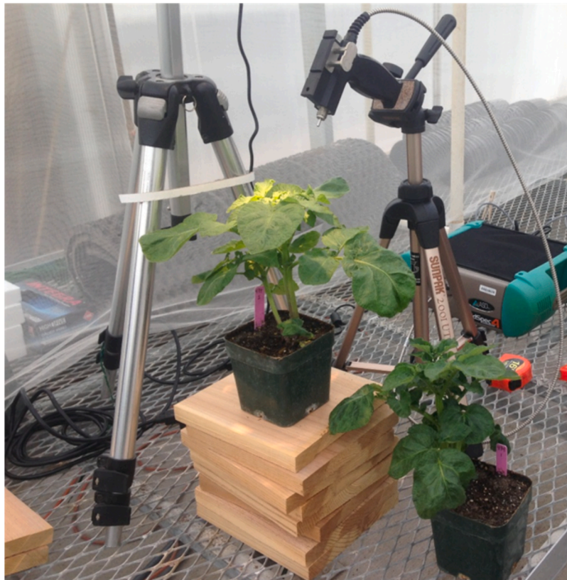
Fig. 2. The field spectrometer equipment setup for data collection in the greenhouse environment.
