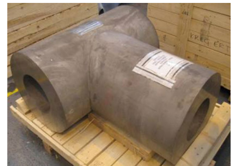
316L PM-HIP component for ASME Section III Code Case N-834 Kyffin, W., Gandy, D., Burdett, B. (2020)
