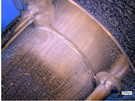
Figure 5. Induction braze of an IN625 sheath instruments and thermowell in a IN625 bulkhead with prototypical thickness to MRTI capsule.
