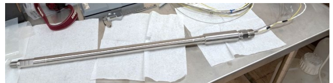
Figure 7. Completed MRTI surrogate salt experiment vehicle.
