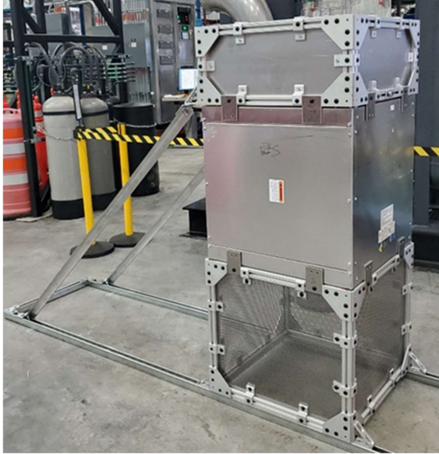
Figure F-3. Photograph of the dilution fan assembly prior to and after installation on the cargo container roof.
