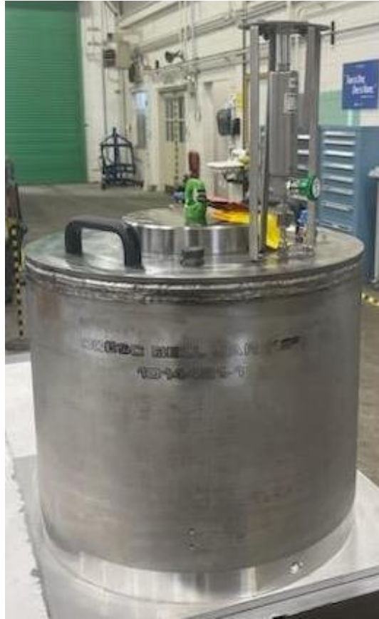
Attachment 1: Photograph of Helium Leak Test Bell Jar assembly (INL Fabrication Work Request 23-151)
