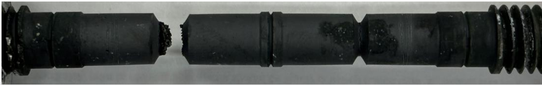
Double V-notch tested until the rupture of one of the V-notches
