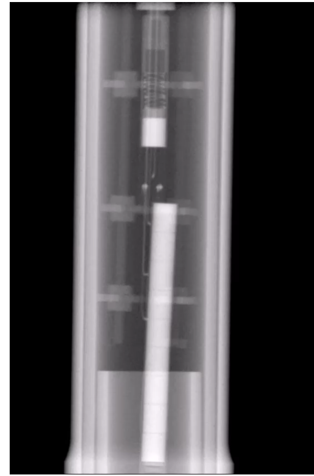
Video of the digital neutron radiographs of SETH-D over the full 360° rotation.
