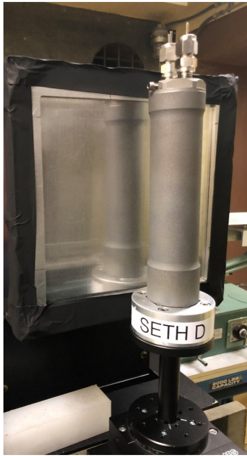
AFTER: (left) Picture of SETH-D experiment mounted in front of the nCT system, (center) example neutron radiograph, and (right) tomographic reconstruction of the SETH-D experiment capsule.
