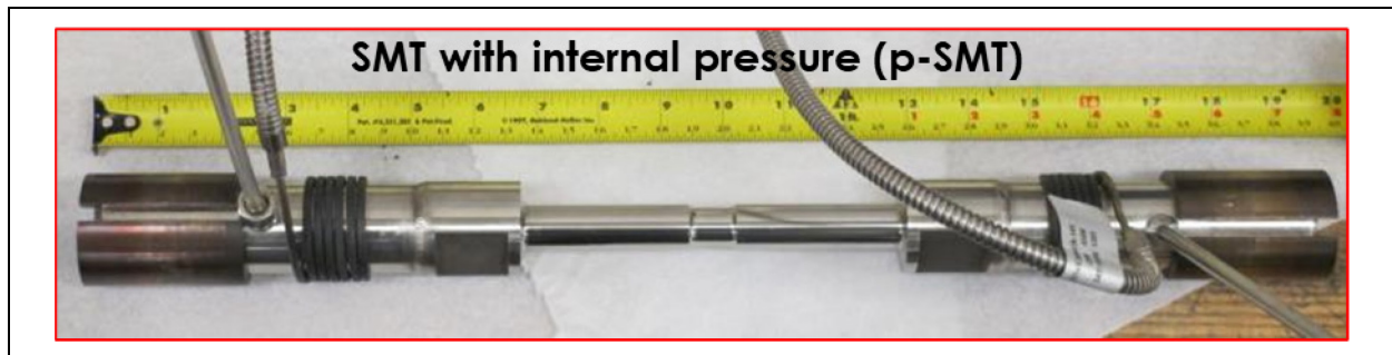
Figure 3. Alloy 617 p-SMT test specimen, photo by ORNL.
