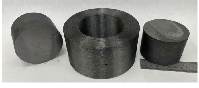
larger tooling, Scale up to experimentation with fiber orientation is underway. 32 mm (left) and 75 mm tooling (right) has been created and tested. Energy savings have been shown to be comparable to that found in the 20 mm tooling comparisons. 150 mm tooling is currently being fabricated.
