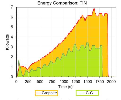
Energy usage with time for samples sintered in C-C tooling, compared to control samples run in identical graphite tooling under identical processing conditions. C-C tooling runs are shorter as a result of faster heating during the warmup step, in which a fixed current is passed through the tooling until it reaches 300 °C. Actual energy usage in kWh is listed in the table below, along with the resultant material properties and the ram temperatures recorded during sintering.
