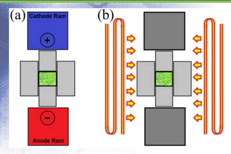
Schematic representations of a) Electric Field Assisted Sintering (EFAS), and b) hot pressing. EFAS uses the tooling itself as the heating element by means of Joule heating as current is passed through the system.
