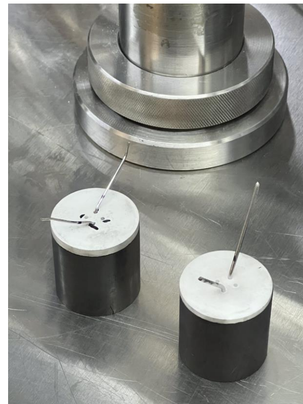
Specimens are setup in crucibles with molten salt, ready for study
