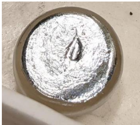
As-cast Fe-Ni alloy immediately after arc melting
