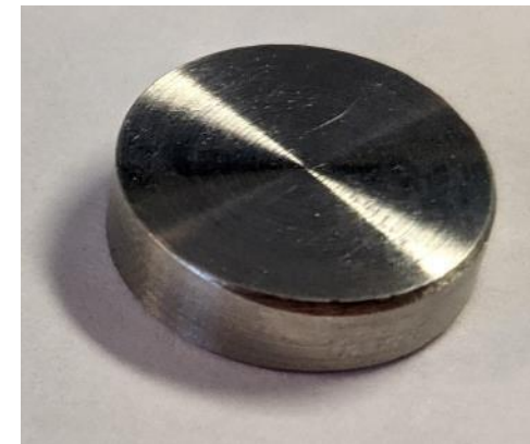
Samples machined to cylindrical geometry with flat & parallel faces
