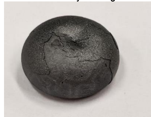
Fe-Ni alloy after annealing at 1100°C for 2 hours, and then naturally cooling
