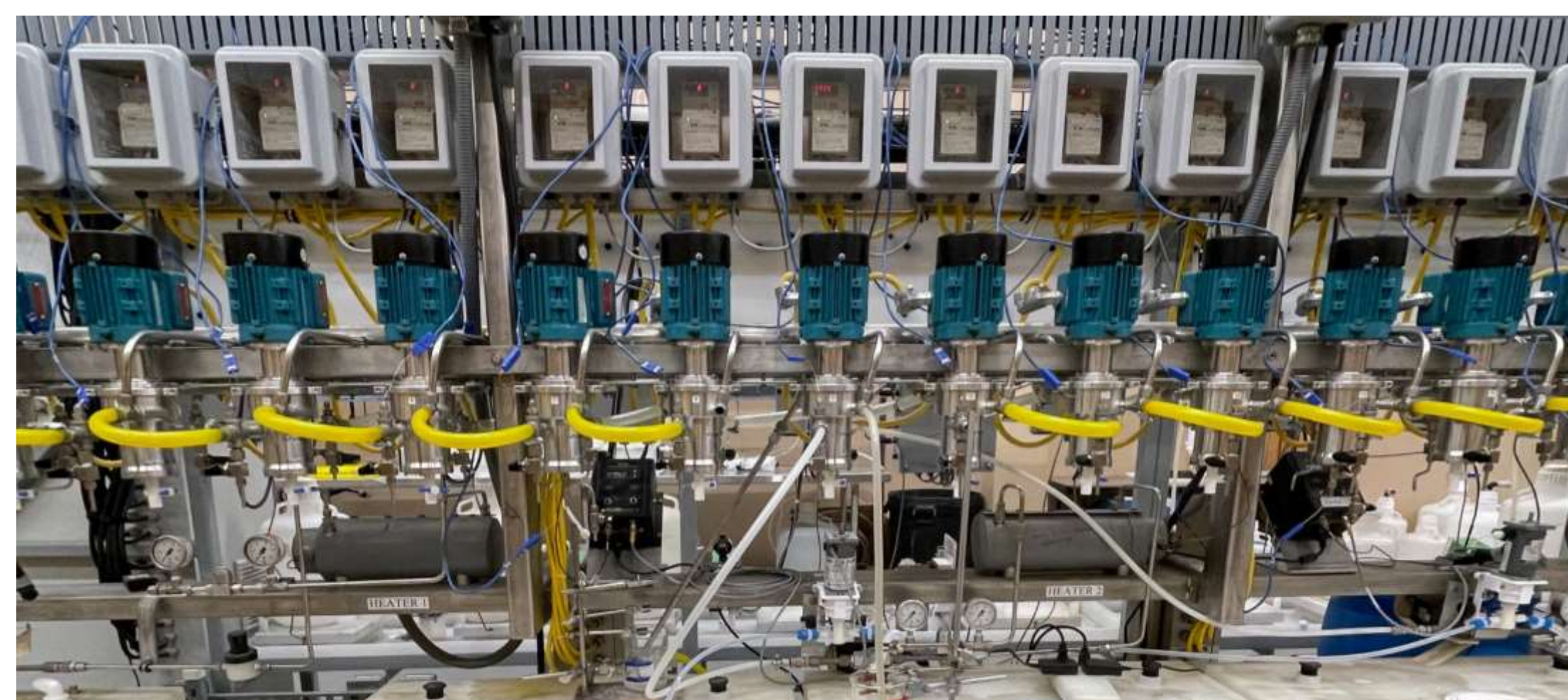
Figure 1. Annular centrifugal contactor array for solvent extraction. The apparatus contains 30 contactors in total, with 8 accelerometers placed on or near the contactors.
